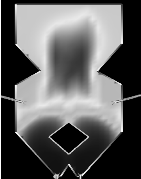
Figure 3. The original picture or boiler area temperatures, generated by linear interpolation of OpenGL quads
